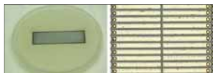
Fig 6 Diamond pixel module prototype: left, a 2 x 6 cm diamond sensor in the wafer for photolithography; right, the 400 micron x 50 micron pixel pads
