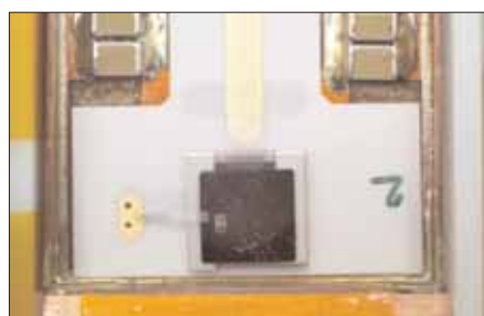
Fig 8 Close up of the diamond sensors – there is a pair of diamonds in each module, one on top of the other
