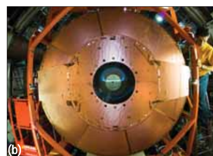
Fig 5 The first ATLAS inner detector with (a) end-cap removed and (b) fully inserted within the liquid argon cryostat
